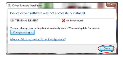
Close this window and open the Device Manager (Computer/Properties/Device Manager). Right click on USB TERMINAL ELEMENT / WERMA MULTICOLOUR BEACON and then click on "Update Driver Software".
